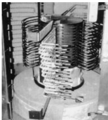
Fig. 6 Overview of the seal-less 30-cell stack
